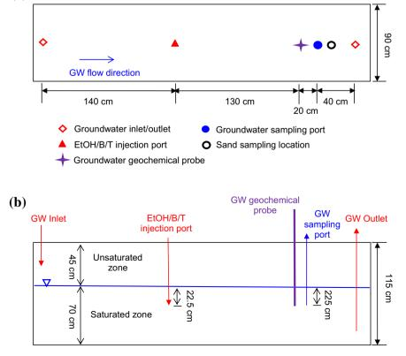
Fig. 1. Plan view (a) and profile view (b) of the pilot-scale aquifer system.
