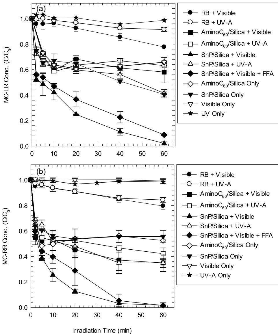
**Fig. 2.** Degradation of (a) Microcystin-LR and (b) Microcystin-RR by sensitizers under UV-A and visible-light irradiation ( $[RB]_0 = 50 \mu\text{M}$ ;  $[\text{aminoC}_{60}/\text{silica}]_0 = [\text{SnP}/\text{silica}]_0 = 0.5 \text{ g/L}$ ;  $[\text{Microcystin-LR}]_0 = [\text{Microcystin-RR}]_0 = 5 \text{ mg/L}$ ;  $[\text{furfuryl alcohol}]_0 = 5 \text{ mM}$ ;  $[\text{phosphate}]_0 = 1 \text{ mM}$ ;  $\text{pH}_i = 7.0$ ).
