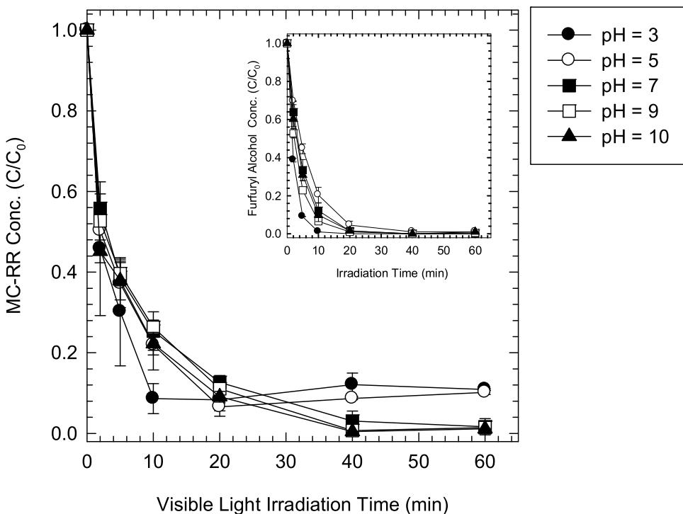
**Fig. 4.** Effect of initial pH on photosensitized degradation of Microcystin-RR by SnP/silica (inset: pH dependence of photosensitized singlet oxygenation) ( $[SnP/silica]_0 = 0.5 \text{ g/L}$ ;  $[Microcystin-RR]_0 = 5 \text{ mg/L}$ ;  $[furfuryl alcohol]_0 = 100 \mu\text{M}$ ).
