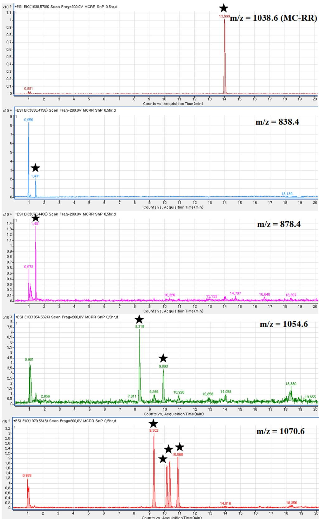
**Fig. 6.** LC/MS chromatograms of extracted ions of Microcystin-RR and its transformation products following treatment with SnP/silica ( $[SnP/silica]_0 = 0.5\text{ g/L}$ ;  $[Microcystin-RR]_0 = 5\text{ mg/L}$ ;  $[\text{phosphate}]_0 = 1\text{ mM}$ ;  $pH_i = 7.0$ , and time = 0.5 h). The peaks with stars indicate the Microcystin-RR and its transformation products whose chemical structures are proposed structures based on their MS/MS spectra (see Figs. S11–S15).
