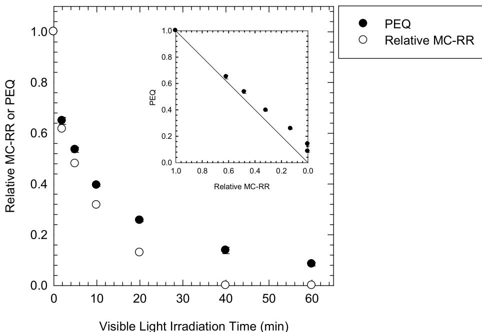
**Fig. 7.** Time-dependent reduction in Microcystin-RR concentration and potency equivalent (PEQ) (inset: plot of PEQ versus relative concentration of Microcystin-RR (i.e.,  $[MC-RR]/[MC-RR]_0$ ) ( $[SnP/silica]_0 = 0.5 \text{ g/L}$ ;  $[Microcystin-RR]_0 = 5 \text{ mg/L}$ ;  $[\text{phosphate}]_0 = 1 \text{ mM}$ ;  $pH_i = 7.0$ ). The solid line represents a perfect negative linear correlation, which indicates that the photosensitized transformation products retain no residual toxic potential.
