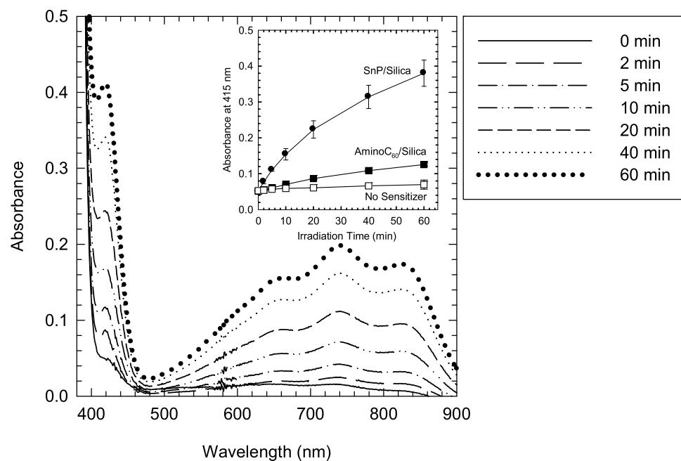
**Fig. 3.** Absorption spectra of ABTS in the presence of SnP/silica as a function of visible light irradiation time (inset: formation of ABTS<sup>+</sup> during the photo-irradiation of SnP/silica and aminoC<sub>60</sub>/silica) ([SnP/silica]<sub>0</sub> = [aminoC<sub>60</sub>/silica]<sub>0</sub> = 0.5 g/L; [ABTS]<sub>0</sub> = 2 mM; [phosphate]<sub>0</sub> = 1 mM; pH<sub>i</sub> = 7.0).
